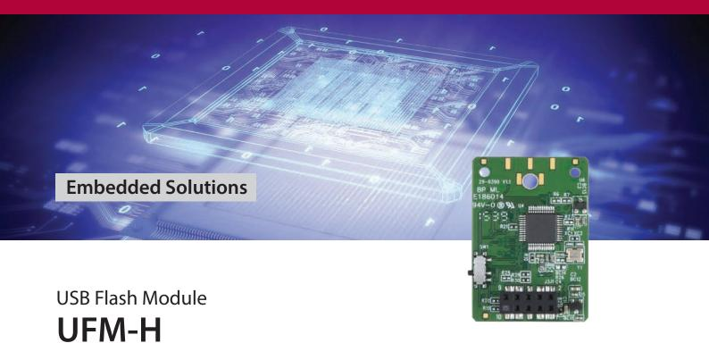
Transcend's USB Flash modules are convenient, easy to implement solutions for expanding the memory capacity of industrial computers. These compact storage devices consume a minimal amount of power and feature a mechanical write protection switch. Due to their minimalist dimensions, these USB modules are suitable for use in small embedded systems.
